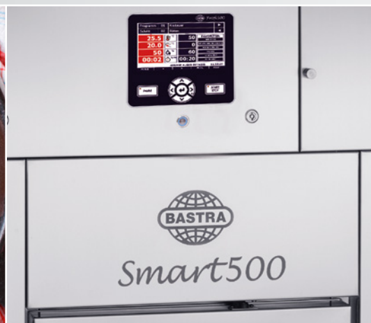
Touchpanel-Steuerung BASTRA Profi500 touchpanel control BASTRA Profi500
