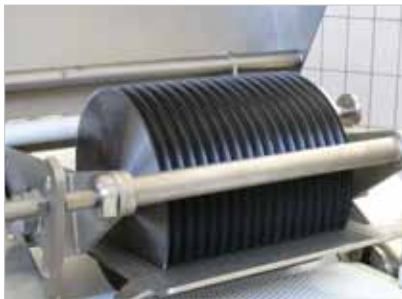
Pict. 1: Example of cutting roller
