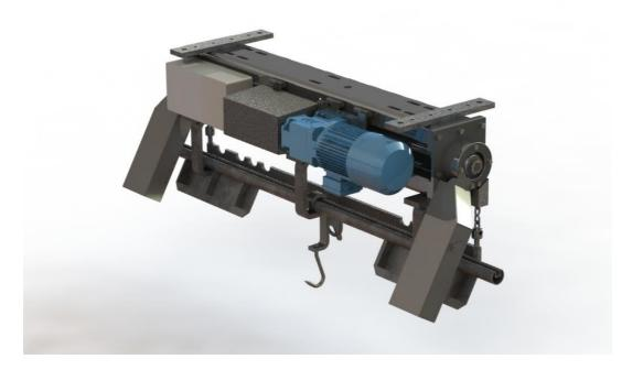
Capacity: Motor: Connection: System protection: Lifting speed: Lifting power: Net weight: Power control: Control system: up to 15 livestock / hr 2.2 kW 3 x 400 V, 5A IP 54 9.6 m / min. 1'400 kg 235 kg UP-DOWN, with EXIT-button Control box with a return stop-and thermal motor protection with limit stop switch for the liftstop
