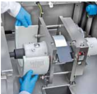
Removal of the evaporation tank for cleaning purposes
