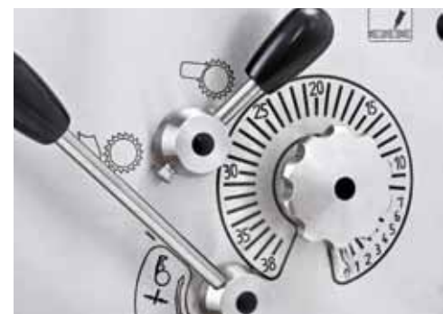
Adjustment wheel for locking individual rind thickness demands.
