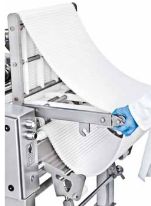
Easy handling of infeed and discharge conveyor belt for cleaning purposes
