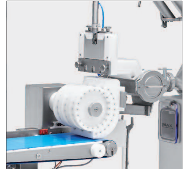
High performance thanks to multi-row form rollers
