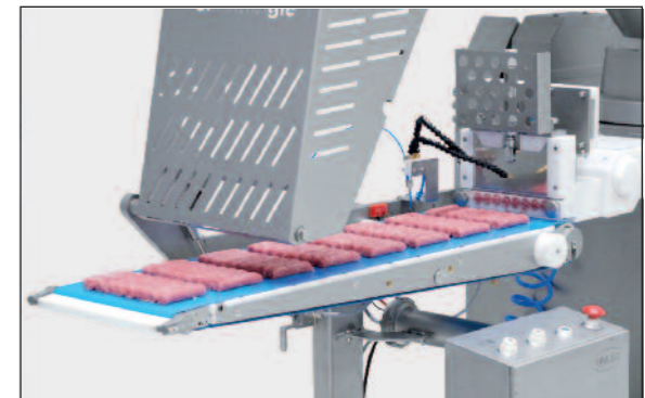
Cevapcici shaping by flow divider & form cutter
