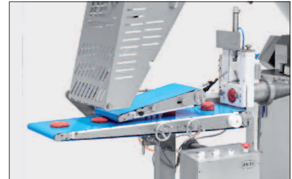
Cevapcici shaping by flow divider & form cutter
